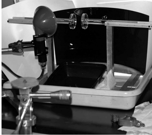
FIGURE 2. Experimental set-up. The strobe light is visible in the foreground. A small amount of the viscous silicone oil is placed between the two vertical disks, which are rapidly pulled apart by rubber bands. A polarizing filter in the background, together with a crossed polarizer on the camera lens, is used to reduce unwanted reflections of the strobe light.
